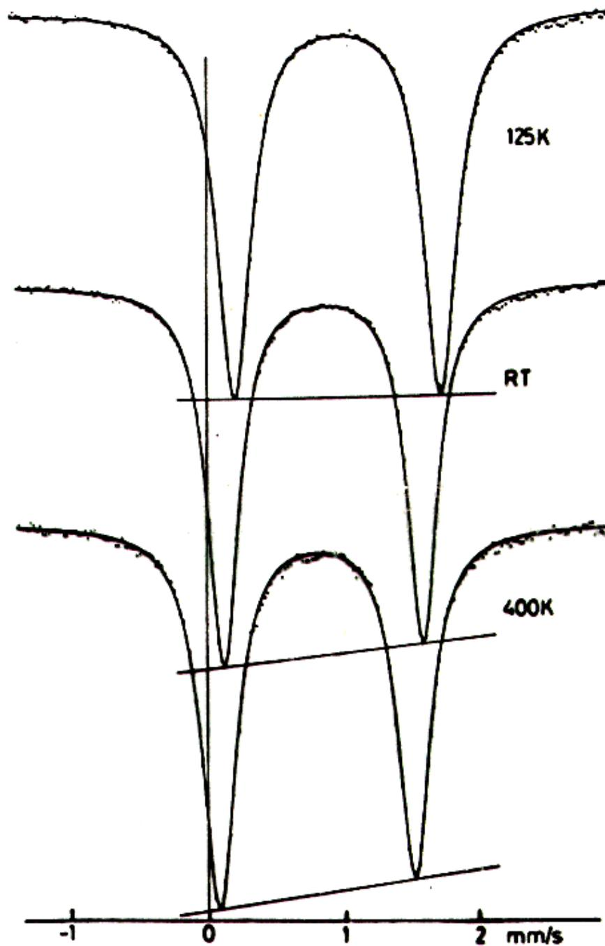
**FIGURE 7.** Mössbauer spectra of FePS, recorded at 125 K, room temperature, and 400 K. The asymmetry is visualized by straight lines through the peak positions (from Reference 38).
