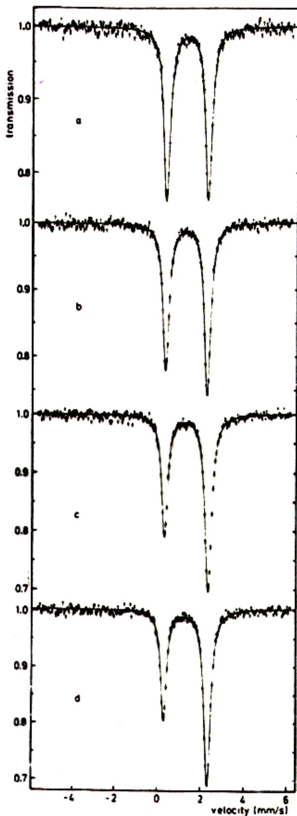
Fig. 3. Temperature dependence of the field-induced asymmetry of the Mössbauer spectrum of polycrystalline FeCO<sub>3</sub> mixed with active carbon powder. (a) Original spectrum at 185 K, (b) spectrum at 185 K after 5 kG at 185 K, (c) spectrum at 60 K after 5 kG at 60 K, (d) spectrum at 60 K after 7.5 kG at 60 K.
