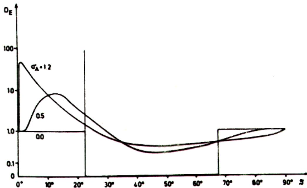
Fig. 6. The texture function  $D_E(\theta)$  calculated with a logarithmic Gauss distribution of the critical field for some values of  $\sigma_A$  and  $a = 0.7056$ . (The ordinate is semilogarithmic so that it is proportional to  $\log(D_E + 0.1)$ .)
