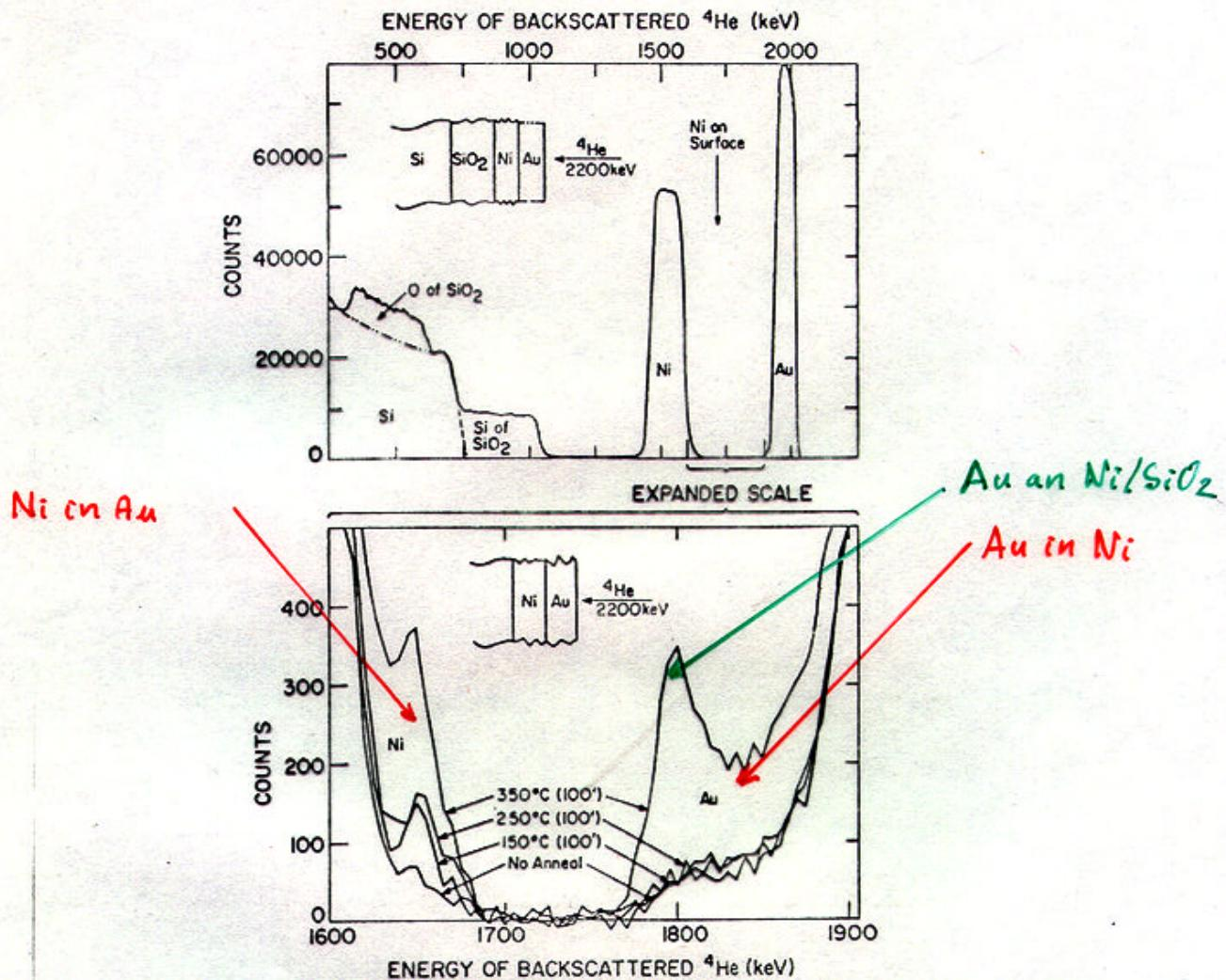
Figure 13) The interdiffusion of two thin metal films is shown for Au and Ni on  $\text{SiO}_2$ . The upper spectrum is from the original target showing the relationship of the various target peaks. Note the Expanded Scale notation (between the Ni and Au peaks) which is shown between the upper and lower drawings. The lower drawing expands this region, and shows superimposed spectra for various heat treated targets. The Ni up-diffusion and the Au down-diffusion are clearly shown.
