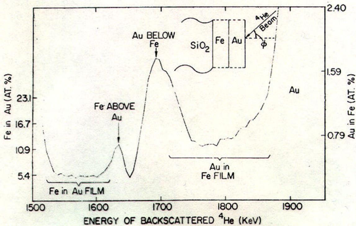
figure 14) By tilting a target of Fe/Au the beam penetrates a thicker target. This expands the region of interest between the two films. The ordinate of the spectrum has been converted to atomic percent of Fe in Au, and Au in Fe, so that concentration profiles can be directly read.
