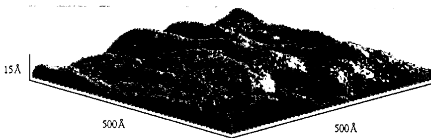
Fig. 1. Three-dimensional shaded view of a 50 nm × 50 nm STM image of nickel evaporated on silicon substrate (as-received specimen).
