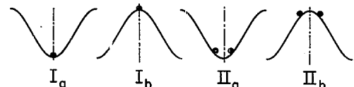
FIG. 17. Atoms at the center of a minimum-energy soliton defect indicating the different symmetry types I_a, I_b, II_a, and II_b . [Compare with Figs. 7(b) and 8(b).]
