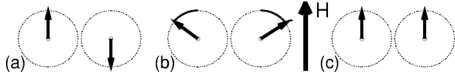
FIG. 1. Basic spin configurations in isotropic antiferromagnetically coupled two-layers ( N=2 ). At zero field (a) the magnetization vectors \mathbf{m}_i are antiparallel in adjacent layers but the structure has no fixed orientation in the plane (infinite degeneracy). An in-plane magnetic field lifts the degeneracy and stabilizes states with \mathbf{l} perpendicular to the field and with \mathbf{m} along the field—this is a spin-flop (SF) phase (b). In a sufficiently strong magnetic field the SF phases transform into the saturated ( flip ) phase (c).
