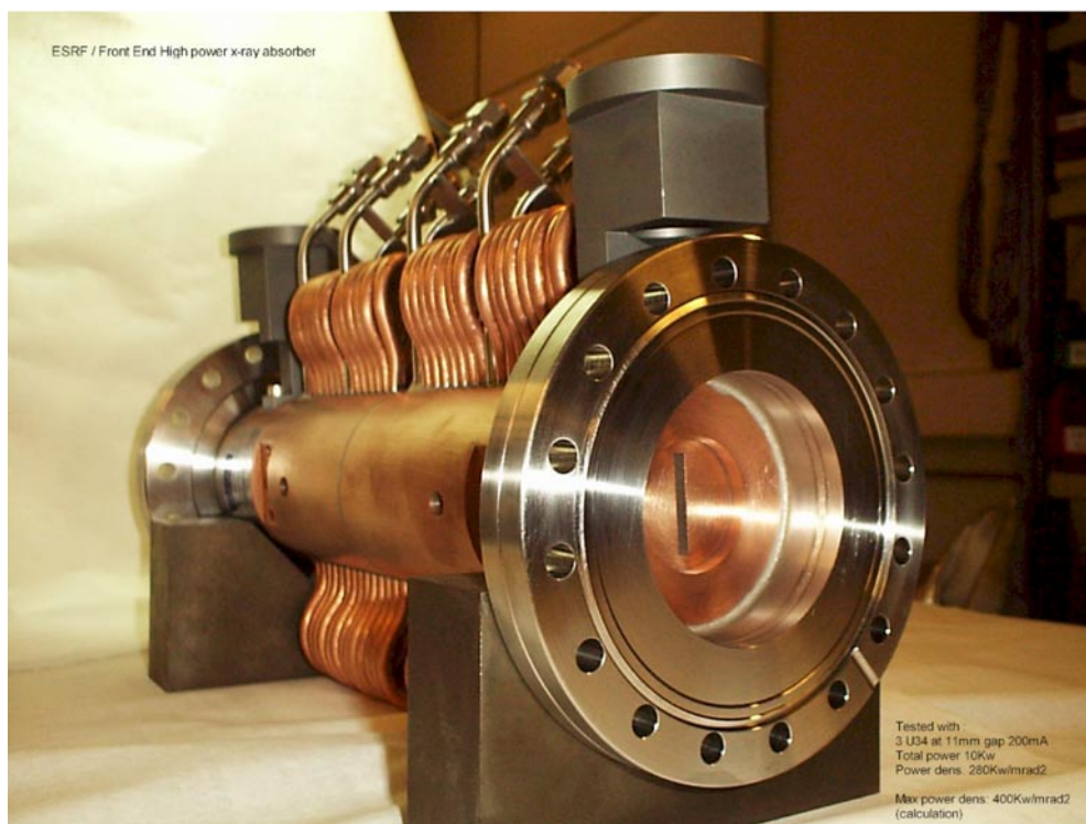
Figure 6. The high power front-end absorber developed at ESRF, which allows us to cool away up to 18 kW of unwanted power, which is emitted off-axis.
