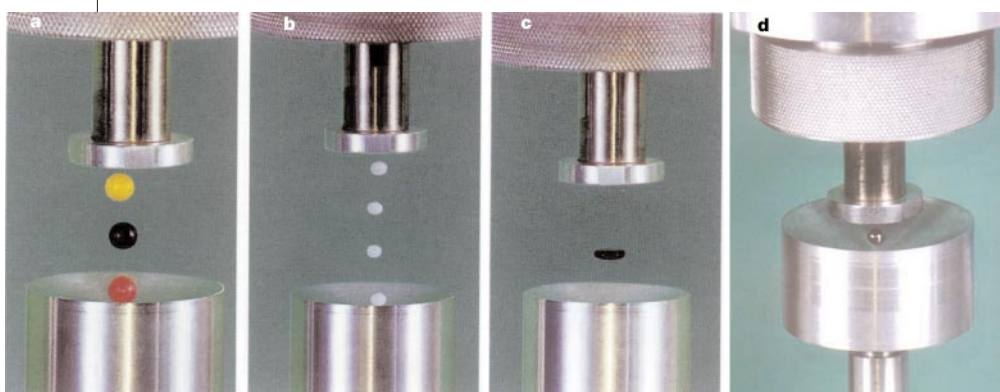
Figure 1 Acoustic levitation by ultrasound. In Xie and Wei's latest experiment 3 the force produced by a standing wave of 16.7-kHz ultrasound, which forms between a vibrating cylinder (top) and a concave reflector (bottom), is enough to levitate small objects. The freely floating objects are: a, three polymer spheres; b, four liquid crystal samples; c, a water drop deformed to a pancake shape by the uneven acoustic pressure; and d, a heavy tungsten sphere levitated in the lowest resonance mode, which has one potential minimum.
